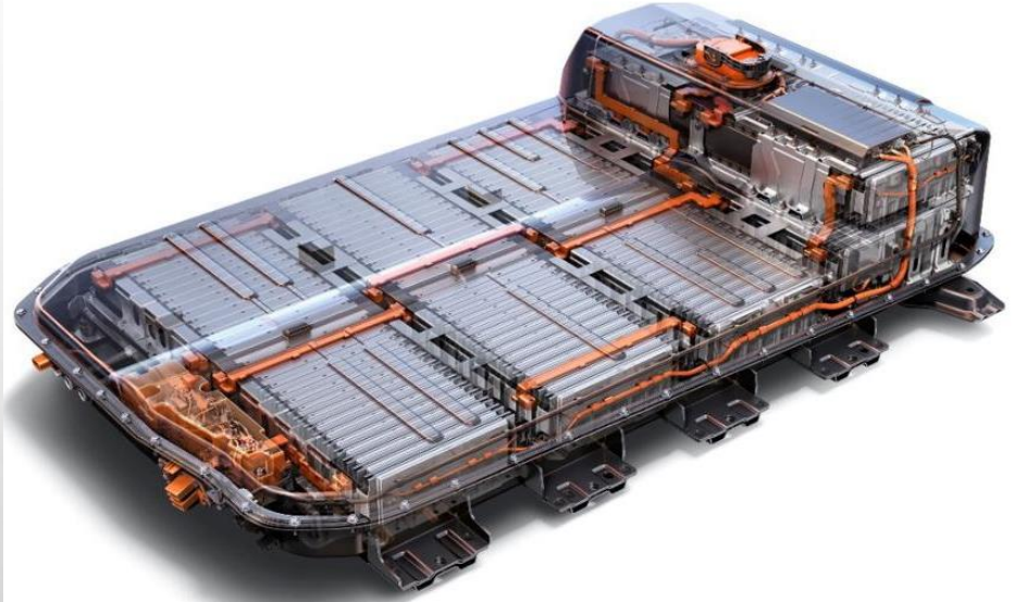
Chevy Bolt Battery Pack is Liquid Cooled via base plate below the cells
