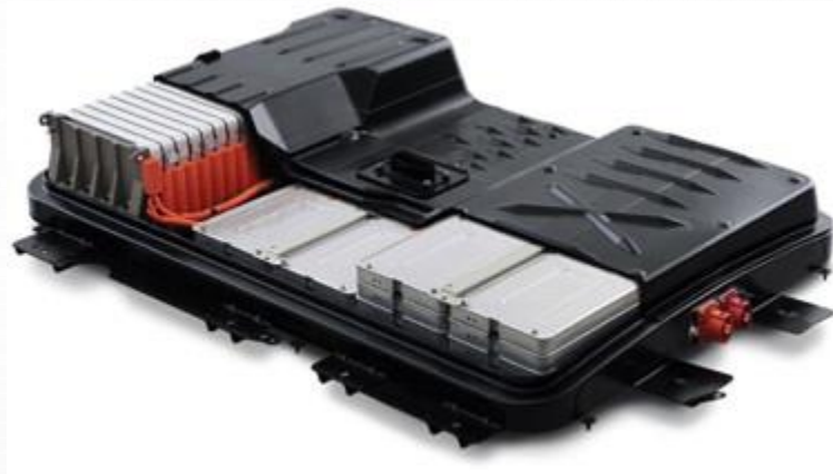
Nissan Leaf – Battery Pack with Air cooling system
